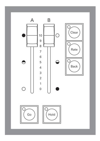
When two scene mode is enabled, the A/B faders control the scenes and function in reverse with respect to each other. When both faders are up, as shown above, fader A is at full and scene A (controlled by the top row of channel sliders) is up on stage. When the faders are both down, fader B is at full and scene B (controlled by the bottom row of channel sliders) is up on stage. Having the sliders function in reverse directions allows for smooth manual crossfades with the use of only one hand.
