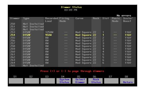
Up to 16 dimmers are shown in the display at once. If a dimmer has an error condition, the entire dimmer row is highlighted in yellow (ordinarily the line is in gray). Dimmer errors are also identified in the About Dimmer display. See *About Dimmer with ETCLink*, page 47.
